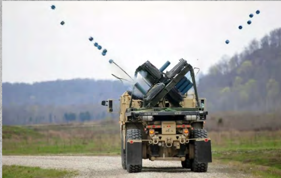
Volcano family of scatterable mines (FASCAM) being delivered from a HEMTT
